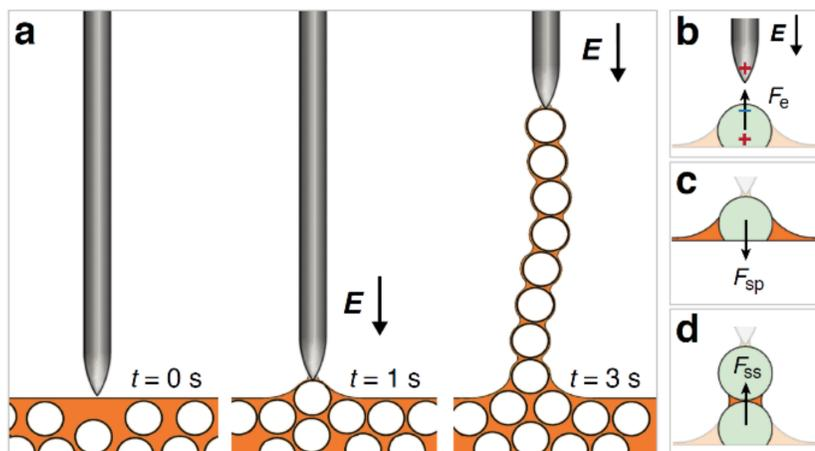
**Fig. 1.** (a) Particles are pulled out of a dispersion to form a 1D structure by applying an electric field through an electrode. (b,c) A particle at the air–liquid interface experiences an upward dielectrophoretic force  $F_e$  and a downward capillary force  $F_{sp}$  stemming from the sphere–plane liquid bridge. (d) Once the particle is pulled out, it automatically forms a sphere–sphere bridge with the particle below it, and pulls that particle upwards with force  $F_{ss}$ .
