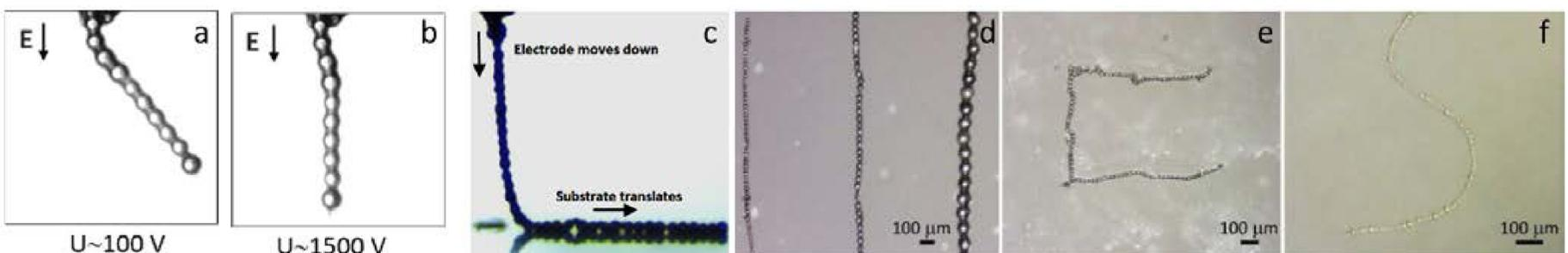
**Fig. 4.** (a,b) A short granular chain, which is actively bent and straightened by changing the magnitude of the applied electric field. (c) Deposition of particles: A particle-chain is formed and then deposited on a substrate that moves horizontally. (d) Example of parallel deposition of chains composed of particles with different sizes, and (e,f) examples of C-shaped and S-shaped pathways.
